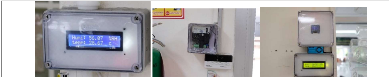
A temperature, light, and humidity control system is in place, divided into zones. (ARU, Thailand)
